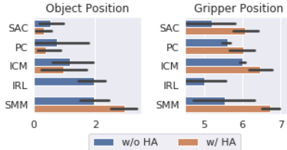
Figure 2.10: With vs. Without Historical Averaging: After training, we rollout the policy for 1e3 epochs, and record the entropy of the object and gripper positions in Fetch . SMM achieves higher state entropy than the other methods. Historical averaging also helps previous exploration methods achieve greater state coverage.
