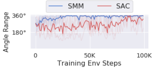
Figure 2.7: Training on Hardware ( D’Claw ): We trained SAC and SMM on the real robot for 1e5 environment steps (about 9 hours in real time), and measured the angle turned throughout training. We see that SMM moves the knob more and visits a wider range of states than SAC. All results are averaged over 4-5 seeds.
