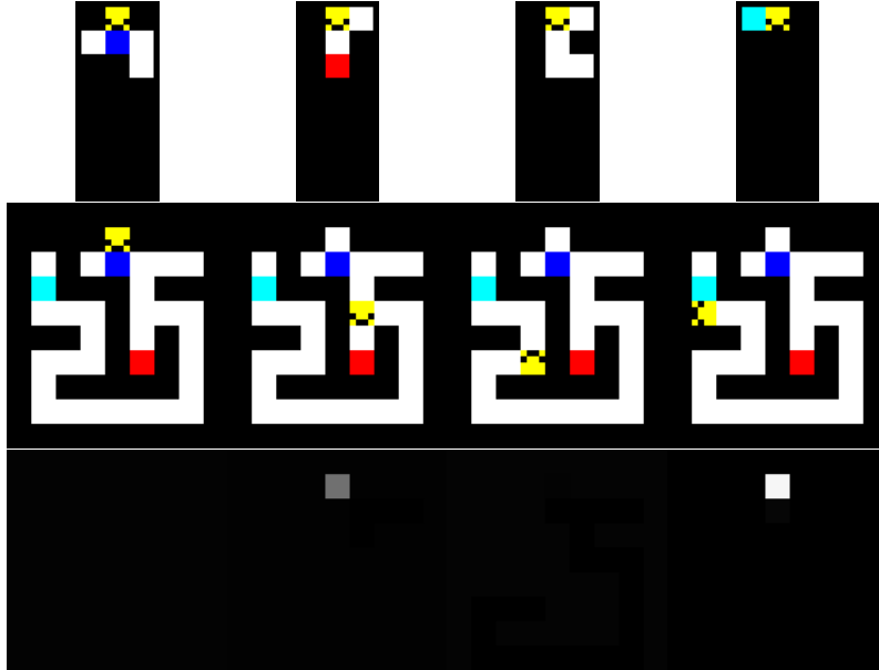
Figure 2.4: A few sampled states from an example episode demonstrating how the agent learns to use the context addressing operation of the Neural Map. The top row of images is the observations made by the agent, the center is the fully observable mazes and the bottom image is the probability distributions over locations induced by the context operation at that step.
