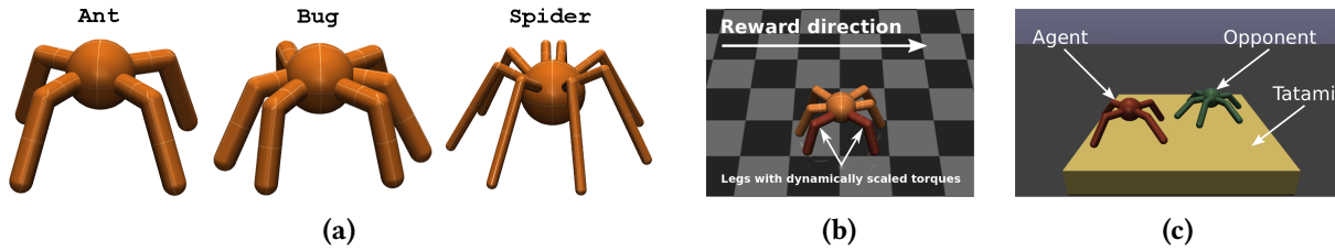
Figure 5.3: Agents and environments used in our experiments. (a) The three types of agents used in experiments. The robots differ in the anatomy: the number of legs, their positions, and constraints on the thigh and knee joints. (b) The nonstationary locomotion environment. The torques applied to red-colored legs are scaled by a dynamically changing factor. (c) ROBOSUMO environment.
